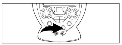
When the vocal feature is activated, the vocals on a multiplex recording are muted as soon as the singer begins singing into the microphone. When the singer stops singing, the vocals are automatically unmuted. Adjust the AVC control for the best balance between playback and microphone levels.
